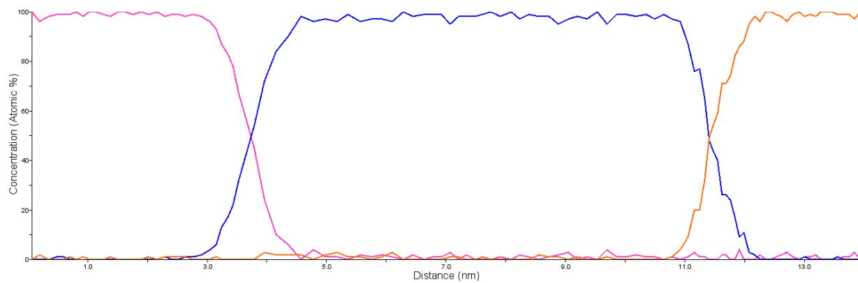
■ Composition plotted vs. distance provides estimates of interfacial chemistry
