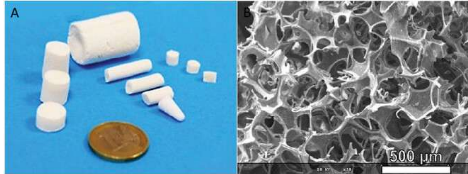
Gelatin/BAG hybrid scaffolds: a) under different shapes; b) observed in scanning electron microscopy. Copyright 2016, The Royal Society of Chemistry (J. Lao, X. Dieudonné, F. Fayon, V. Montouillout, E. Jallot, J. Mater. Chem. B2016, 4, 2486)
