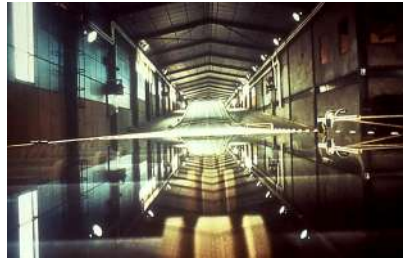
Glass ribbon produced with the float glass process
