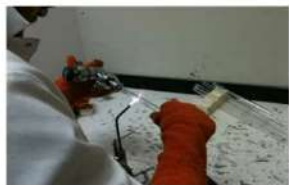
Seal ampule while under vacuum with an O 2 /CH 4 torch
