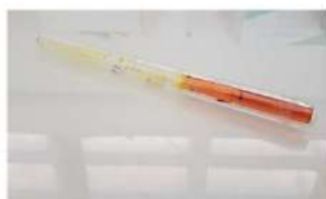
Seal ampule while under vacuum with an O 2 /CH 4 torch
