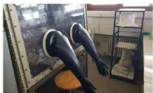
Batch in a glove box from elemental Ge, Sb, S and Na 2 S
