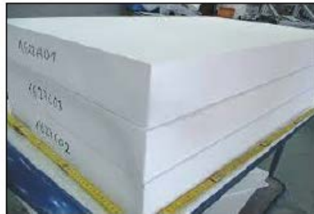
Insulating ceramic plates made of alumina (thickness : 100mm) [M. Schumann & L. San-Miguel, 2017]
