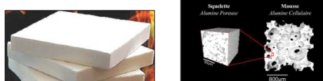
NorFoam sample [Saint-Gobain Refractories website] NorFoam Xpure microstructure [PhD thesis, Z. K. Low, 2016, INSA Lyon]
