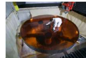
→ telescope mirror Very Large Telescope (VLT - Eso) Zerodur® (Schott)
