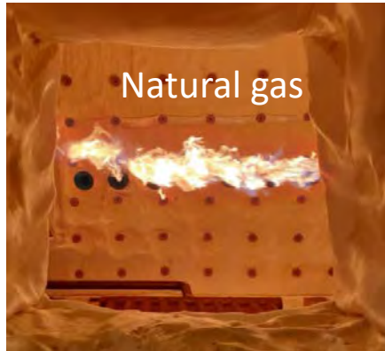
Observation at 200KW CF burner in NG-Mode
