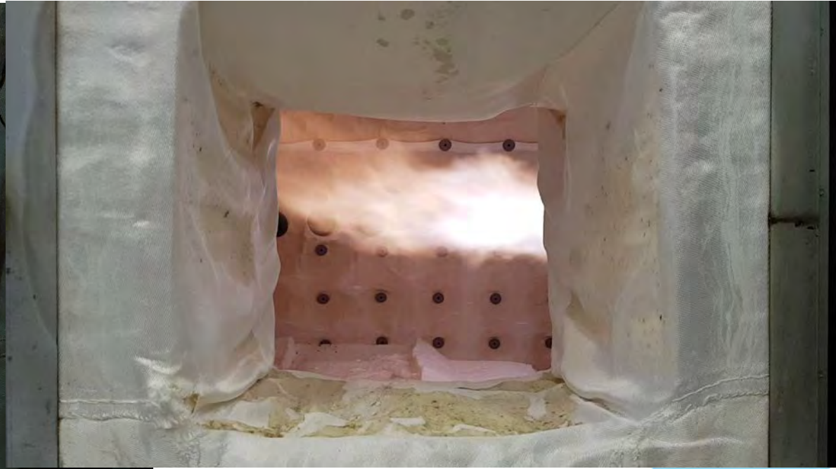
Observation at 200KW CF burner in HYDROGEN-Mode
