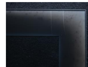
Lack of scratch resistance
