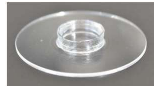
Fig. 5. Printed quartz glass cylinder with a diameter of 20 mm and 10 overlying glass layers, P = 120 \text{ W} , f_{\text{rot.}} = f_{\text{adv.}} = 250 \text{ mm/min} , \rightarrow \rightarrow .
