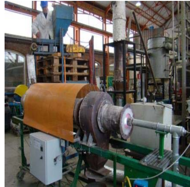
Rotary furnace: direct heating
