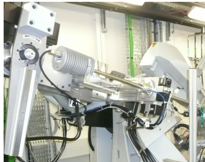
SDD detector mounted on the 2θ arm.
