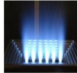
Submerged burner for heating & pollutions digestion
