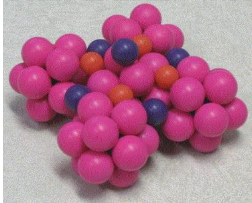
Interpenetrating clusters in the **efficient cluster packing model** of Miracle et al.
