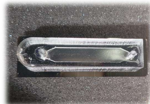
PDMS fluidic cells are bounded to control the interaction length
