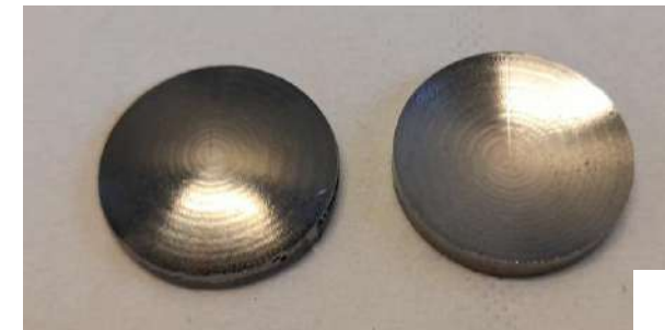
High-index IR lenses that can be integrated into automotive devices
