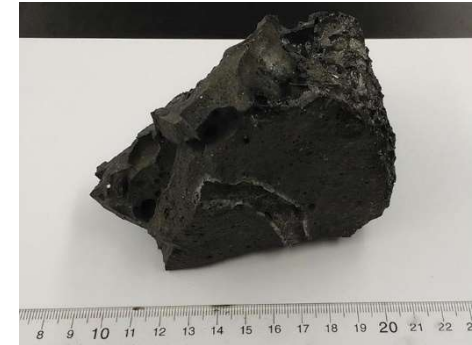
iron phosphate waste form containing 40 wt% of simulated nuclear waste. https://mo-sci.com/
