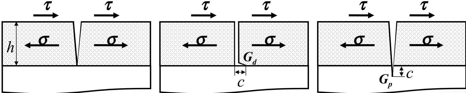
$G_d$ : driving force for debonding along the interface
