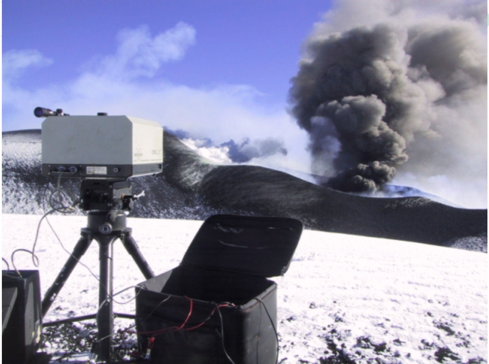
FTIR measurements of the emissions from the 2750 m. a.s.l. cone during the 2002 eruption of Mount Etna (Courtesy of Mike Burton, INGV Catania).
