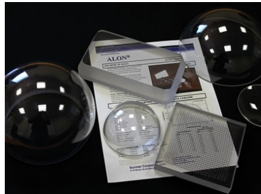
ALON Infrared windows optical lenses [1]
