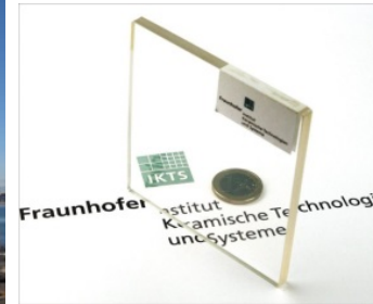
\text{MgAl}_2\text{O}_4 Transparent armor [2]
