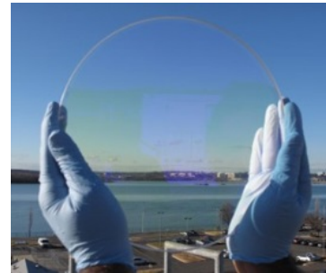
\text{MgAl}_2\text{O}_4 Transparent armor [2]
