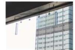
Developed glass antenna that adds cellular base station capabilities to windows
