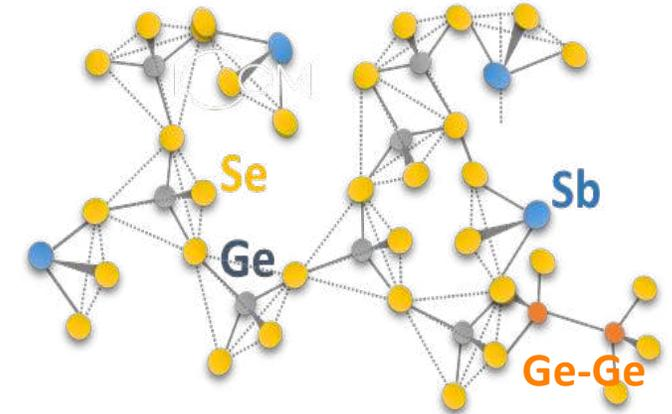
Structure of thin film closer to bulk glass at higher pressure ( $[\text{GeSe}_{4/2}]$  tetrahedra,  $[\text{SbSe}_{3/2}]$  pyramids)
