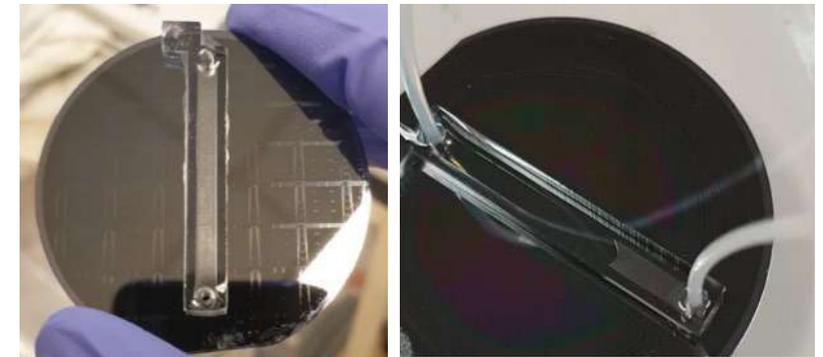
PDMS microfluidic device grafted onto the microstructured chalcogenide substrate and PIB polymer coating filled with water
