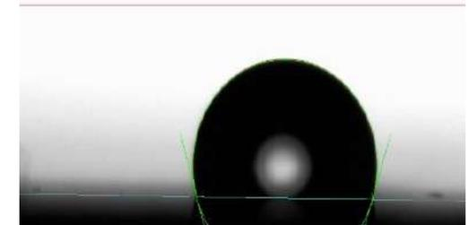
Contact angle measurement close to expected value (100-110°)
