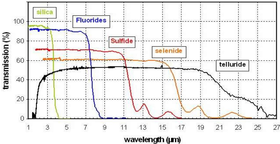
Selenide glasses present broader transmission window in IR than sulfide
