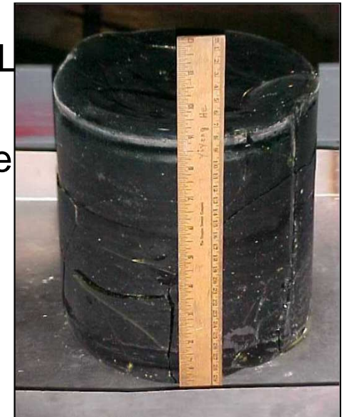
Simulated waste glass cylinder, 8 liters, melted at 1200°C (Brow, personal communication)
