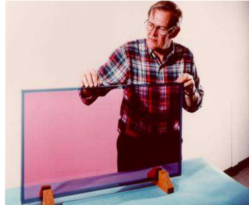
Beamlet eighteen liter rare earth doped phosphate glass amplifier slab
