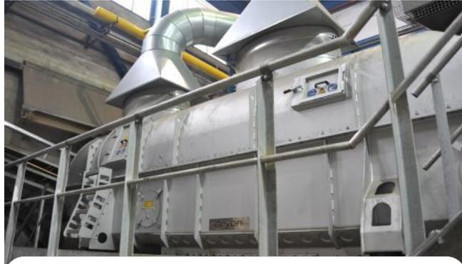
:: Efficient drying of glass cullet, extraction of fine waste particles
