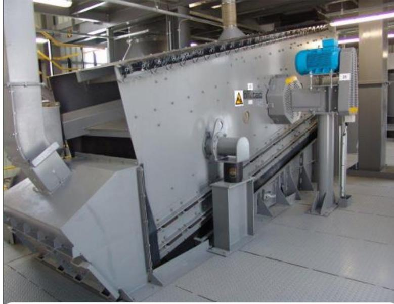
:: Specific screening and preparation for the sensor based sorting
