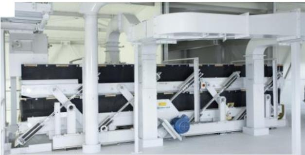
:: Coarse fractionation in combination with wind sifting
