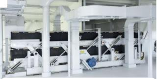
:: Coarse fractionation in combination with wind sifting
