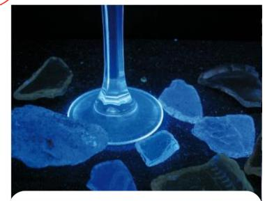
:: Optical sorting system for separating lead glass (containing lead with up to 0,5% PbO concentration) by fluorescence technology - without X-Ray
