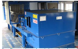
:: Removing aluminium (and copper, ...) pieces (more than 4 mm)
