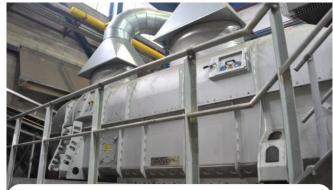
:: Efficient drying of glass cullet, extraction of fine waste particles With Fluidized bed dryer
