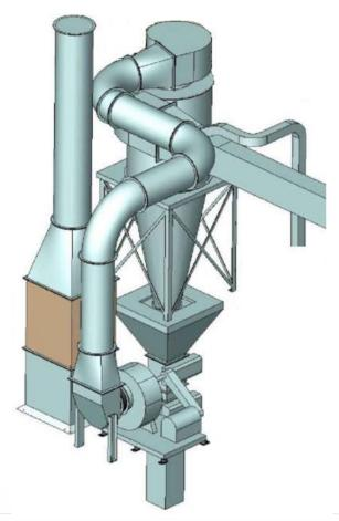
:: Removing paper and plastic (light fraction) with suction
