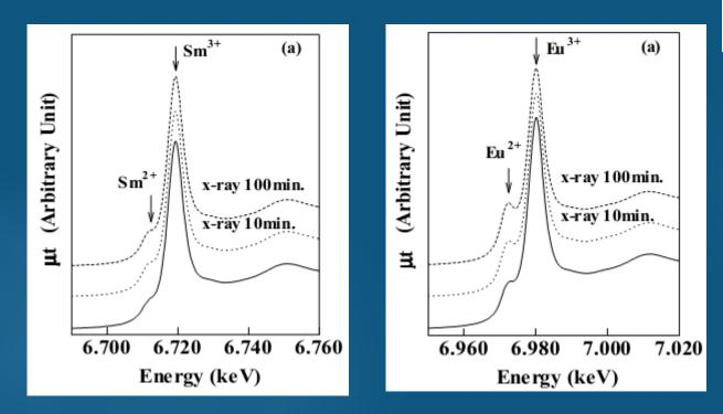
X-ray induced reduction of rare earth ion doped in Na,O-AI,O ,-B,O, glasses
