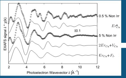
Strong similarity with simulated spectra of  $Er_{Ca}^{\bullet}$  or  $2Er_{Ca}+V_{Ca}$ .
