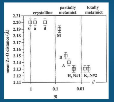
**First shell Zr-O** Reduction of the NN Shrinking of the bond length
